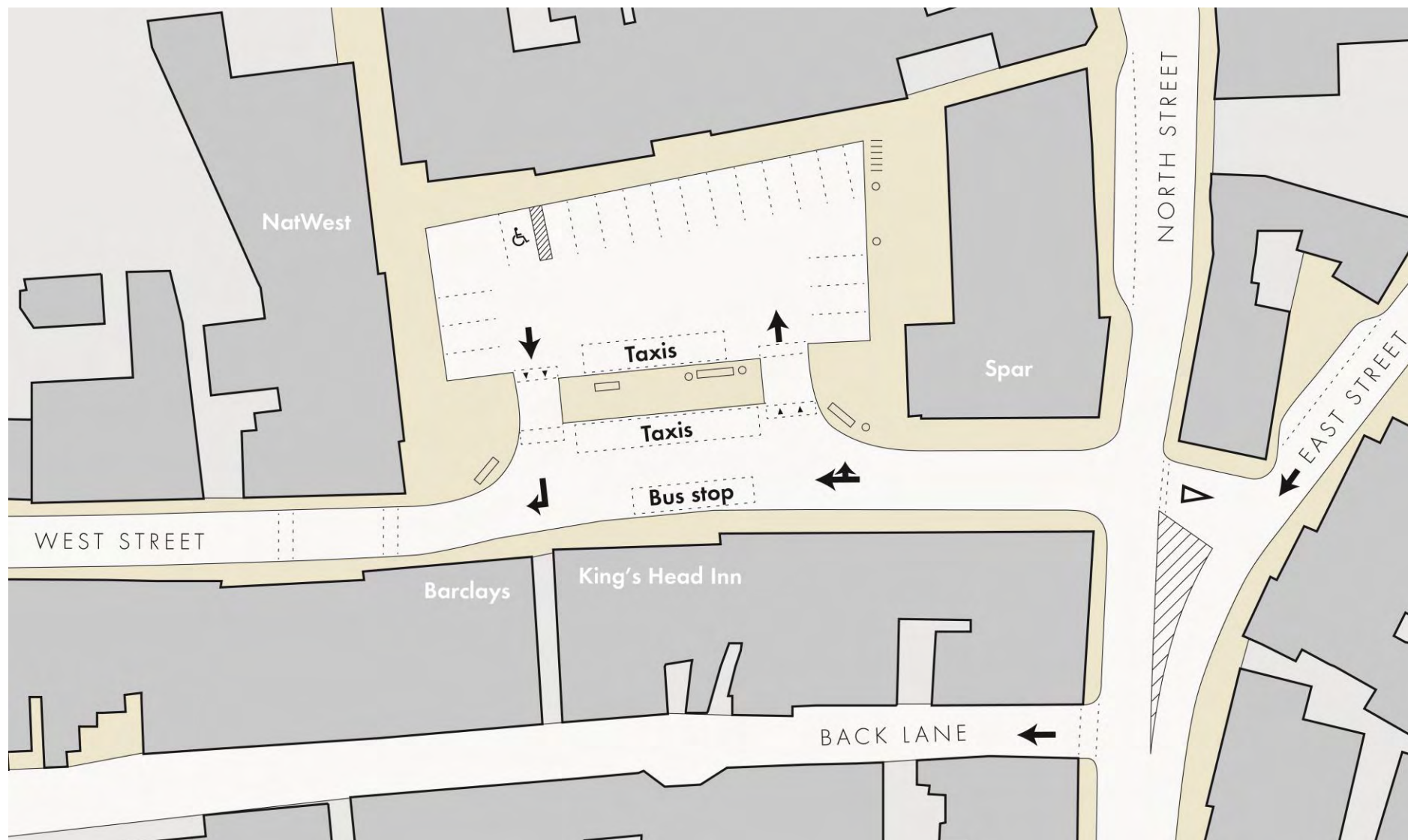
Figure 10 – Market Square existing – plan showing the existing traffic management arrangements within the Market Square with 18 car parking bays (one disabled), four taxi bays and one bus stop
